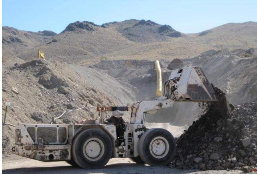
Figure 4. Loader stock piling “Discovery Zone” high-grade at portal of decline
